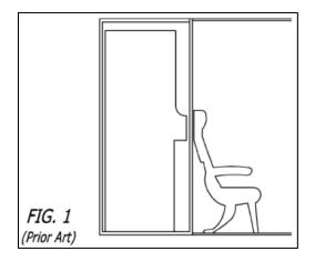
A person of ordinary skill in the art would realize that when such a seat is moved further aft, the first component to impact the wall is the seat back. Ex. 1004, ¶189. As explained above, Betts includes a forward facing recess that receives the seat back. *Id*.
