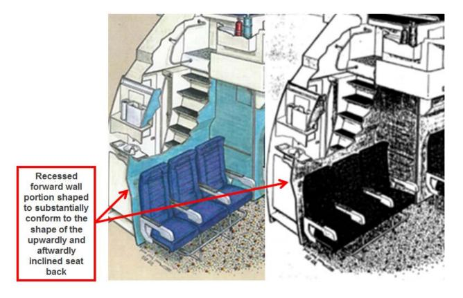
['641 Claim 1 Element C] further includes a second recess configured to receive at least a portion of the aft-extending seat support therein when at least a portion of the upwardly and aftwardly inclined seat back of the passenger seat is received within the first recess.
