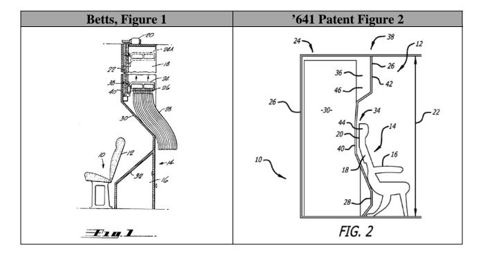
['641 Claim 1 Element B] wherein said forward wall portion is shaped to substantially conform to the shape of the upwardly and aftwardly inclined seat back of the passenger seat, and includes a first recess configured to receive at least a portion of the upwardly and aftwardly inclined seat back of the passenger seat therein, and
