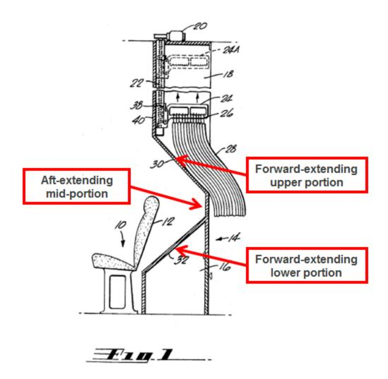
['641 Claim 16] The aircraft lavatory according to claim 8 wherein said first aft-extending recess extends along substantially a full width of said forward partition.
