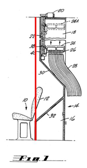
['641 Claim 10] The aircraft lavatory according to claim 9 wherein said forward -extending upper portion is configured to project over at least a portion of the forward-positioned passenger seat.
