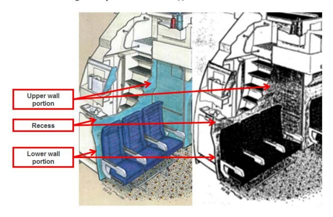
['641 Claim 8, Element C] wherein the forward-extending upper portion, the aft-extending mid-portion, and the forward-extending lower portion combine to define a first aft-extending recess disposed between the upper forward-extending portion and the forward-extending lower portion, and
