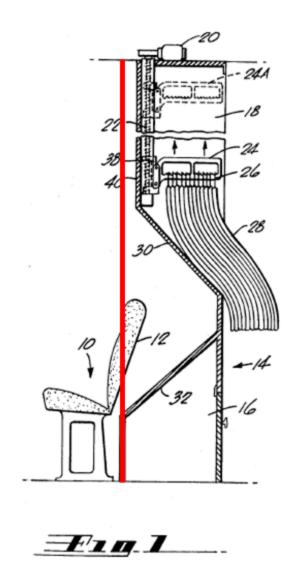
One of ordinary skill in the art would understand that the forward wall of the enclosure shown in Betts would also be suitable for use with other aircraft enclosures, including lavatories. Ex. 1004, ¶59. In an aircraft, as a row of seats is moved further aft, the first thing that would make contact with a flat wall is the top of the back of the seat. Ex. 1004, ¶59. And so Betts includes a recess that receives that portion of the seat back. Applying the contoured wall of Betts to a lavatory
