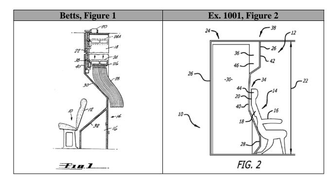
['641 Claim 15] The aircraft lavatory according to claim 8 wherein the upper forward-extending portion, the aft-extending mid-portion, and the forward-extending lower portion of the forward partition form a substantially continuous surface.
