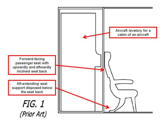
As explained in Section V above, a person of ordinary skill in the art would be motivated to modify a flat wall lavatory to use the KLM Crew Rest design on the forward wall of a lavatory. The KLM Crew Rest document shows a side elevation of a lavatory enclosure. Ex. 1004, ¶175. The enclosure has a contoured
