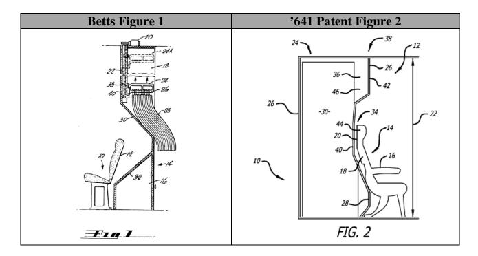
['641 Claim 1 Element C] further includes a second recess configured to receive at least a portion of the aft-extending seat support therein when at least a portion of the upwardly and aftwardly inclined seat back of the passenger seat is received within the first recess.
