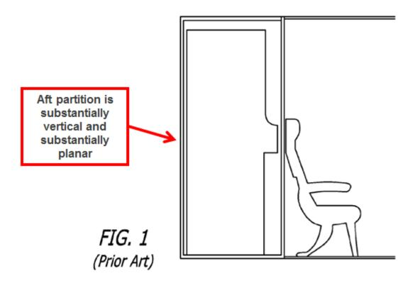
['641 Claim 14] The aircraft lavatory according to claim 8 wherein the width of the lavatory space disposed between the forward partition and the aft partition comprises an upper width, a lower width, and a mid-width, and wherein the upper width and the lower width are both substantially wider than the mid-width.
