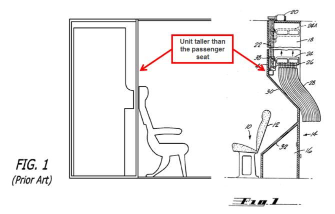
['641 Claim 5] The aircraft lavatory of claim 1, wherein said forward wall portion includes a lower portion that is disposed under the passenger seat back when at least a portion of the upwardly and aftwardly inclined seat back of the passenger seat is received within the first recess and at least a portion of the aft-extending seat support is received within the second recess.
