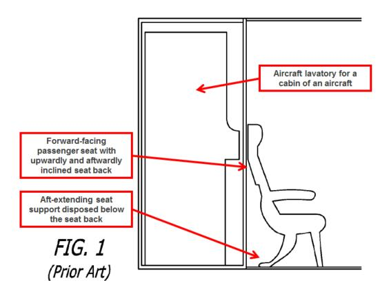
['641 Claim 1 Element A] a lavatory unit including a forward wall portion and defining an enclosed interior lavatory space, said forward wall portion configured to be disposed proximate to and aft of the passenger seat and including an exterior surface having a shape that is substantially not flat in a vertical plane;
