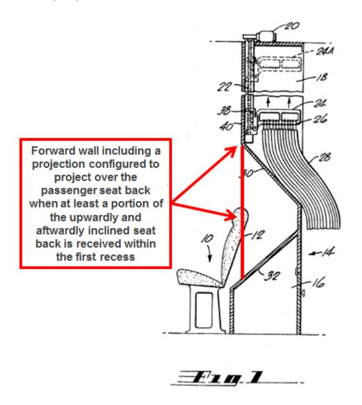
Further, as explained above with regard to *Claim 1, Element C*, a person of ordinary skill in the art would be motivated to modify a flat forward wall to include a second recess to receive at least a portion of an aft extending seat support. Ex. 1004, ¶196. One motivation for such a modification would be to allow for the seat to be positioned further aft in an airplane cabin. *Id*.
