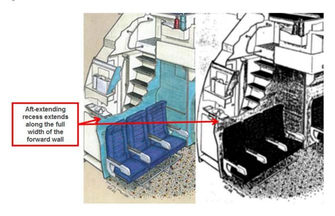
['641 Claim 17] The aircraft lavatory according to claim 8 wherein said lavatory has a top, a bottom, a height therebetween, and a middle therebetween, said lavatory has varying lengths along the height of the lavatory, and said lavatory is longer at the top of the lavatory than at the bottom of the lavatory.
