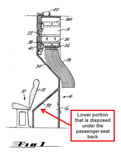
Further, as explained above with regard to *Claim 1, Element C*, a person of ordinary skill in the art would be motivated to modify a flat forward wall to include a second recess to receive at least a portion of an aft extending seat support. Ex. 1004, ¶196. One motivation for such a modification would be to allow for the seat to be positioned further aft in an airplane cabin. Ex. 1004, ¶201.
