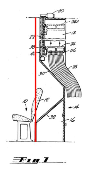
As explained in Section V above, a person of ordinary skill in the art would be motivated to modify a flat forward facing wall of a lavatory to include a recess to allow a passenger seat to be positioned further aft in the aircraft cabin. Ex. 1004, ¶188. Adding a second recess is no less obvious than adding the first recess. A seat with an aft extending seat support is well known in the art. *See, e.g.*, Ex. 1001, Figure 1.
