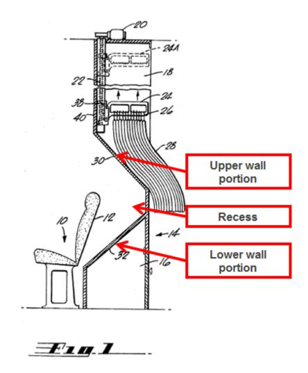
['641 Claim 8, Element C] wherein the forward-extending upper portion, the aft-extending mid-portion, and the forward-extending lower portion combine to define a first aft-extending recess disposed between the upper forward-extending portion and the forward-extending lower portion, and
