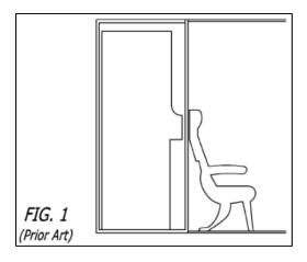
A person of ordinary skill in the art would realize that when such a seat is moved further aft, the first component to impact the wall is the seat back. Ex. 1004, ¶217. As explained above, the KLM Crew Rest document includes a forward facing recess that receives the seat back. *Id*.
