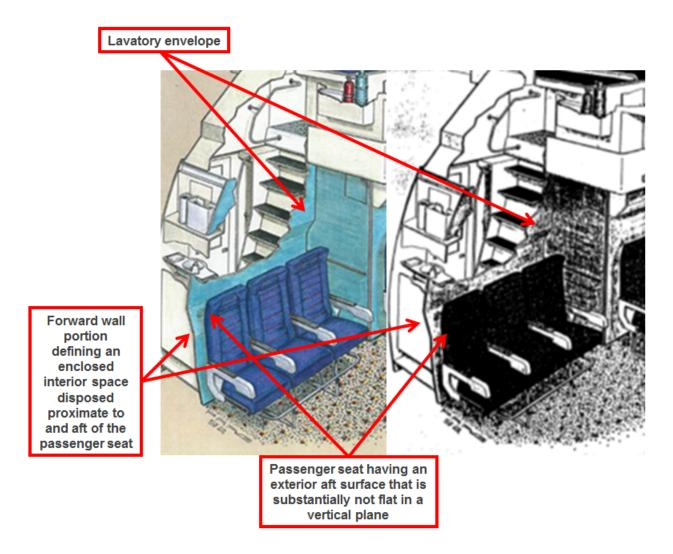
The contoured forward wall includes an exterior surface having a shape that is substantially not flat in a vertical plane.
