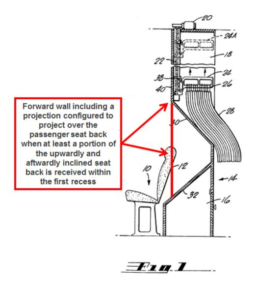
['641 Claim 12] The aircraft lavatory according to claim 9 wherein said lavatory is taller than the forward-positioned passenger seat.
